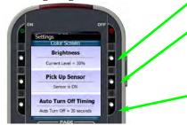
Adjust the brightness of the screen to taste. In most lighting conditions, 50% gives good results.
